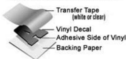
**Transfer Tape** - use to hold the decal together.
